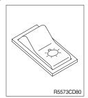
(1) This switch use to operates the head light and work light by two step.
